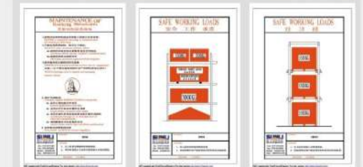
安全標識 Signs containing basic safety data and recommended loading limits should be prominently displayed within the operating area of the racking
