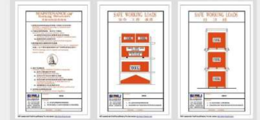
安全標識 Signs containing basic safety data and recommended loading limits should be prominently displayed within the operating area of the racking
